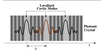
**Figure 1.** Schematic drawing of a coupled optical microcavity structure. A highly localized cavity mode interacts weakly with the neighbouring cavity modes, and therefore the electromagnetic waves propagate through coupled cavities.
