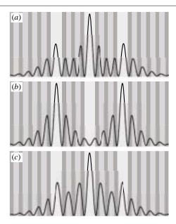
**Figure 4.** Calculated field patterns of three coupled cavities for the resonant wavelengths (*a*)  $\lambda = \lambda_1$ , (*b*)  $\lambda = \lambda_2$  and (*c*)  $\lambda = \lambda_3$ . These modes can be constructed by the superposition of the individual cavity mode which is localized at each cavity site.
