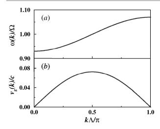
**Figure 6.** (*a*) Calculated dispersion relation of the CMC structure by using equation (8) with  $\kappa = -0.07$ . (*b*) The group velocity is plotted according to equation (9) as a function of wavevector *k*. The group velocity is one order of magnitude smaller than the speed of light at the band centre ( $k\Lambda = \pi/2$ ), and vanishes at the band edges ( $k\Lambda = 0$  and  $\pi$ ).
