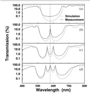
**Figure 2.** Measured (solid curves) and calculated (dotted curves) transmission spectra for (*a*) a DBR and (*b*) single-cavity, (*c*) two-coupled-cavity and (*d*) three-coupled-cavity structures. Due to coupling between the strongly localized microcavity modes, the single-cavity mode splits into two or three distinct modes depending on the number of coupled cavities. There is a good agreement between the measured and the calculated transmission spectra.
